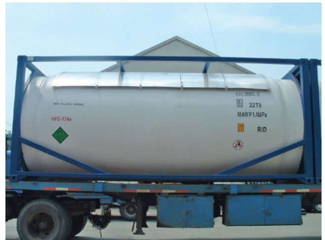
Refrigerants gas tank container
